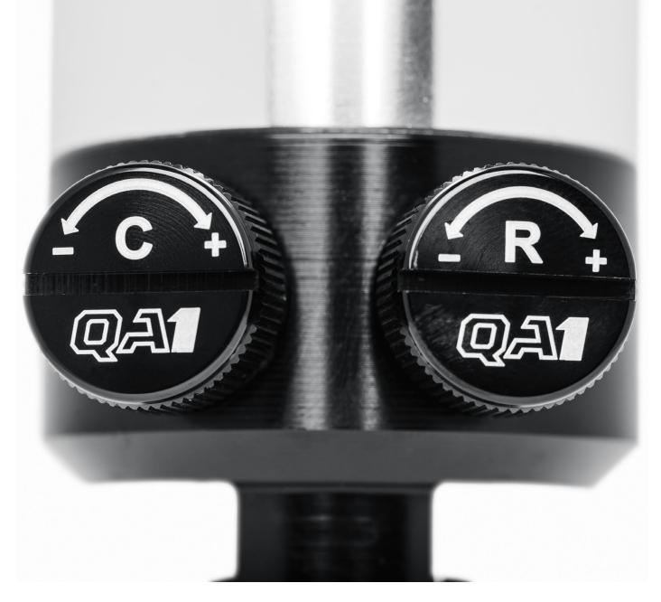
In terms of performance and application, single adjustable shocks are suited for moderate performance enhancements, balancing ease of use with improved handling characteristics. They are ideal for enthusiasts seeking a straightforward upgrade. Double adjustable shocks, on the other hand, provide maximum performance enhancement through precise tuning, essential for applications where handling and stability are critical. They are best suited for high-performance and competitive environments.
