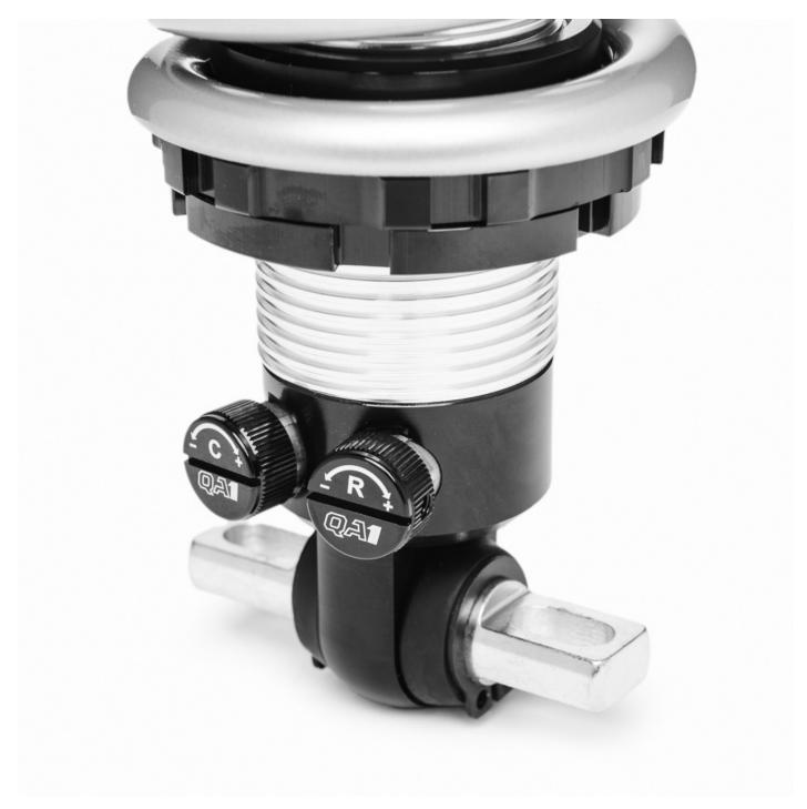
The ability to adjust compression and rebound damping independently means that double adjustable shocks can significantly enhance handling and stability. This versatility makes them highly adaptable to various applications, from street driving to professional racing. The precise control over suspension dynamics also helps achieve an optimal balance between ride comfort and handling performance.
